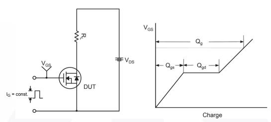
Figure 14. Gate Charge Test Circuit & Waveform
