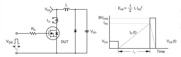
Figure 16. Unclamped Inductive Switching Test Circuit & Waveforms
