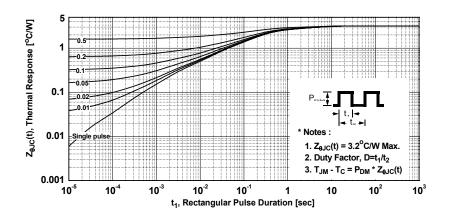
Figure 13. Transient Thermal Response Curve - FDP12N60NZ
